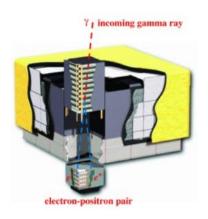
The Fermi LAT is a <u>pair conversion detector</u> on board the Fermi Gamma-Ray Space Telescope.
