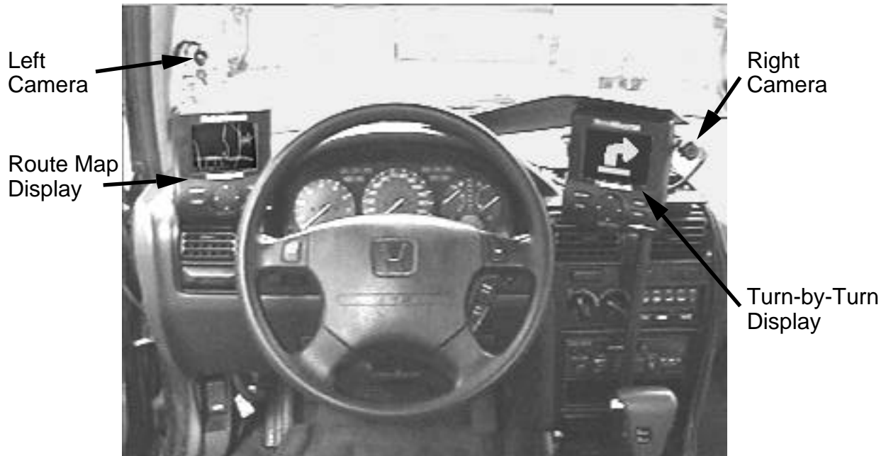
Figure 2. Drivers' dashboard view. Note: the location of the turn-by-turn and route map displays was counterbalanced between subjects.
