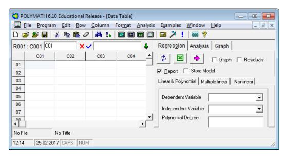
Before inserting the data into the spreadsheet, it is recommended to change the column name with the name of the variable mentioned in the data table. This would make it easy to comprehend the polymath output. To change the column name of C01, double click on the column name "C01" or right click on C01 and select "Column Name..." A dialog box will appear where column name can be changed
