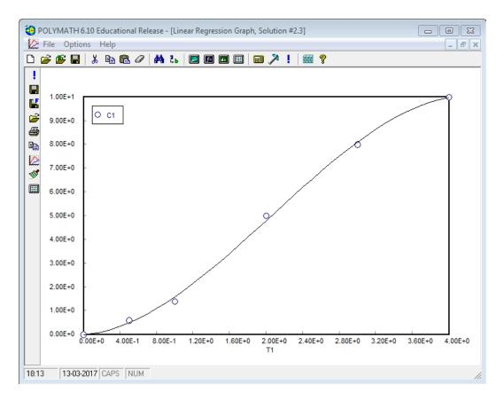
To enter the second set of data in the spreadsheet, change C03 to T2 and C04 to C2, enter the data in corresponding column and then you need to select the dependent and independent variable as C2 and T2 from the drop down menu (shown by red circle in the screenshot). Select the polynomial degree as 3 as was done earlier. Your window will appear like this
