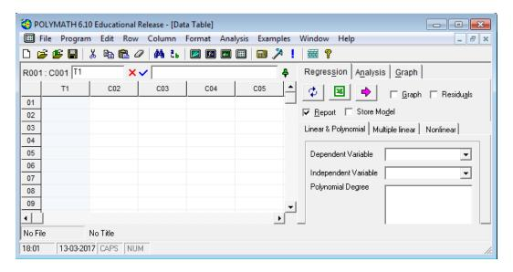
Similarly, rename C02 to C1 as shown below. By default Polymath select Regression method as "Linear and Polynomial". If it is not so, then, click on the Regression tab on the right side of the window, and select the "Nonlinear" regression tab under the "Report" and "Store Model" check boxes (shown by red rectangle) The window should look like this:
