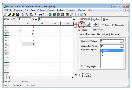
You can also change the dependent variable, independent variable by selecting from the drop down menu next to variable name. In this case we want to change the polynomial degree only. Let's try to fit the data by Polynomial degree 3. Select the Polynomial degree as 3 as shown below
