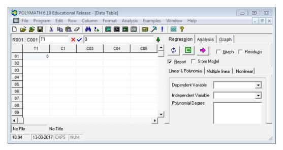
Similarly, enter the remaining data of T1 in subsequent rows. Repeat this procedure to input the data for C1. After entering the data, the spreadsheet would look like this
