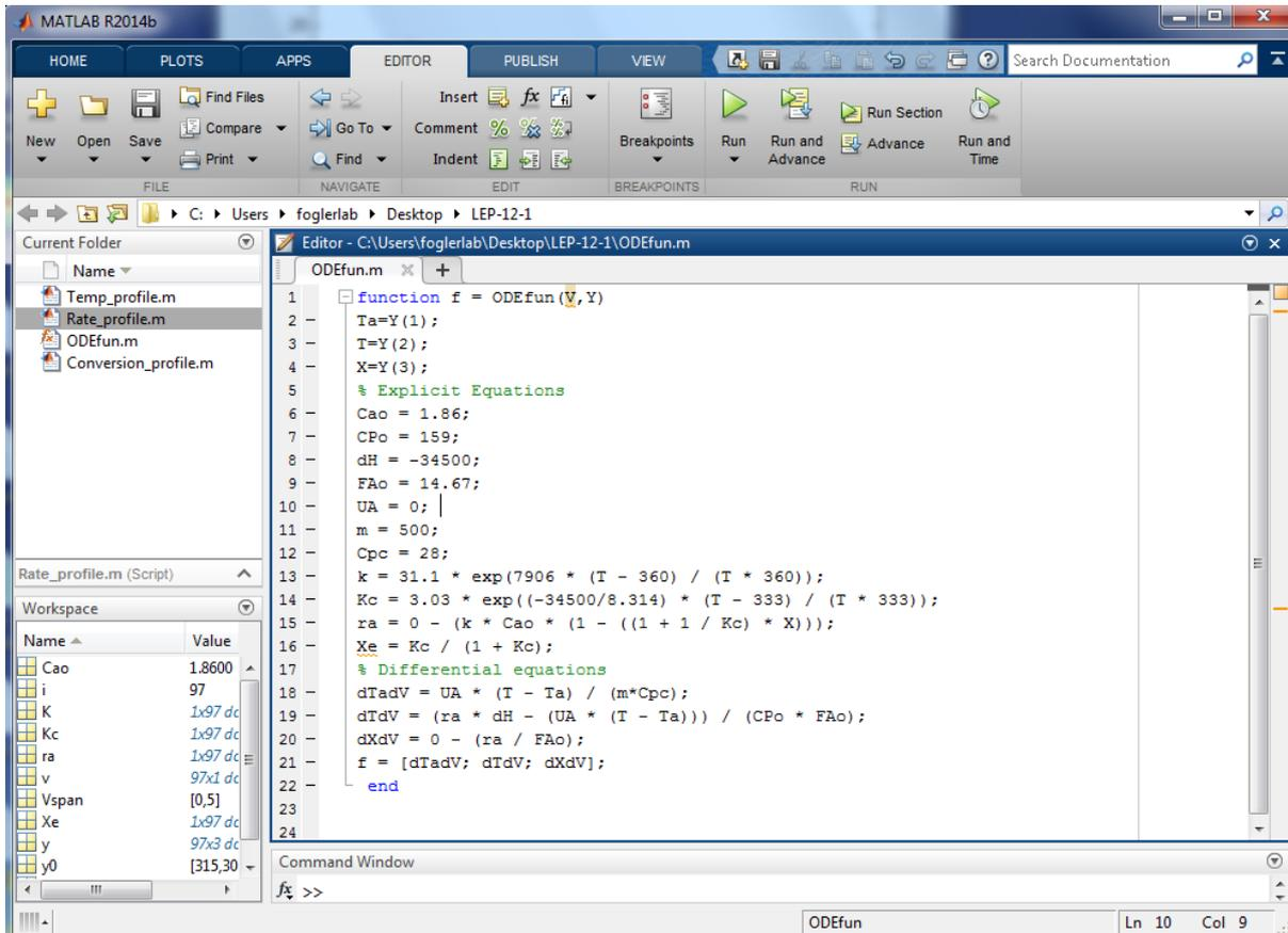
The screenshot shows the MATLAB R2014b Editor window. The current folder is 'C:\Users>foglerlab\Desktop>LEP-12-1'. The workspace contains variables: Cao (1.8600), i (97), K (1x97 dc), Kc (1x97 dc), ra (1x97 dc), v (97x1 dc), Vspan ([0,5]), Xe (1x97 dc), y (97x3 dc), and y0 ([315,30]). The ODEfun.m file is open, showing the following code:
