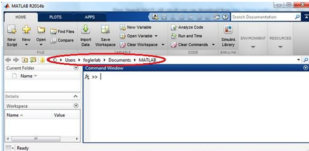
The central window is called Command window. In the command window you can enter statements, run your files, generate output etc.
