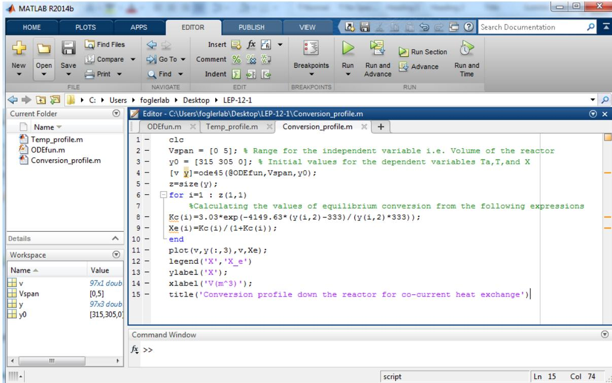
**Step 21:** Now run the conversion file either by clicking run button or typing “Conversion\_profile” and pressing enter in command window. The following graph will be generated
