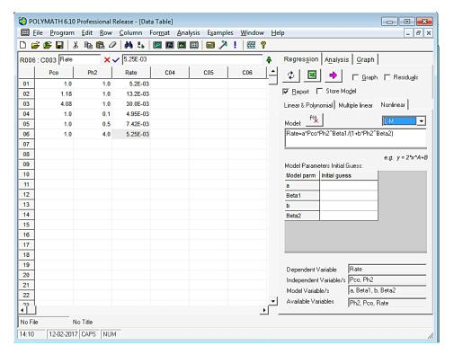
Next we need to select an appropriate regression analysis routine. To select, click on the drop down menu present over the top right of the rectangular box as shown and select the regression method. In this case, we have chosen "L-M".
