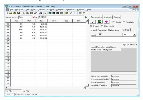
Now, you need to input the model form you wish your equation to match. In this case, the form is Rate=a\*Pco\*Ph2^Beta1/(1+b\*Ph2^Beta2), where Pco,Ph2 and rate are columns in the data table that we are using.
