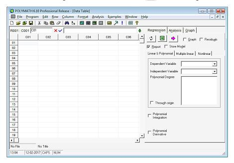
Before inserting the data into the spreadsheet, it is recommended to change the column name with the name of the variable mentioned in the data table. This would make it easy to comprehend the polymath output. To change the column name of C01, double click on the column name "C01" or right click on C01 and select "Column Name..." A dialog box will appear where column name can be changed
