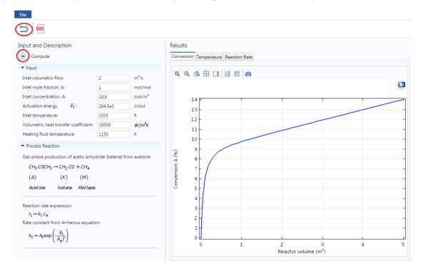
**Step 10:** Now let's consider a case where you want to maintain the Inlet concentration such that 100 % conversion is achieved at the end of the reactor. Enter the inlet concentration of A as 50 mol/m<sup>3</sup> and click compute to see its effect on profile.
