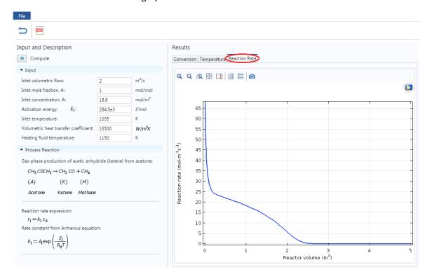
**Step 7:** Under Input section on the left hand side, you can view and change any parameter values. Let's change a parameter and see the effect on the profile. Change the Temperature of heat exchanger medium from 1150 K to 900 K. After you are done, click on Compute button (=) present above the Input parameters
