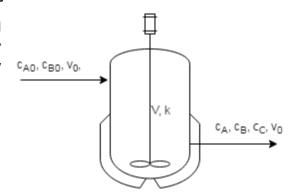
The volumetric flow of reactants is  $v=v_0=0.5\frac{m^3}{s}$  and the active volume of the reactor is  $V=1000m^3$ .
