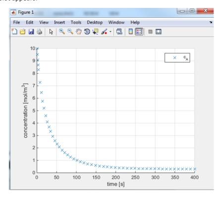
We analyze the solution: at time 0 the concentration of Species A is equal to 10 mol/ $m^3$  and gradually decays until the steady state is achieved (around 250 seconds after the onset of the reaction). You can play with parameters (especially k, V and  $v_0$ ) to see which of them has the largest impact on the shape of the curve. What is the conversion of A (complete/incomplete) at the steady state for different set of parameters?
