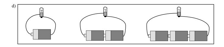
Abdul used a brightness meter to test the brightness of light bulbs in different circuits. In each circuit, he used <u>new</u> batteries and the same type of light bulb.
