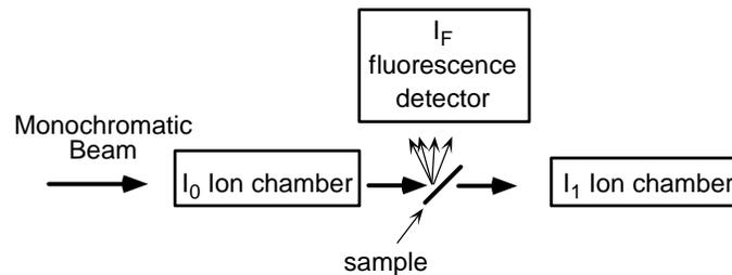
Measure fluorescence intensity as excitation energy is scanned
