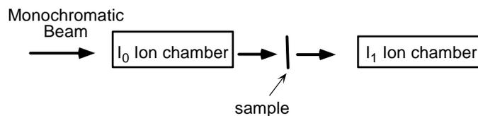
$$A = \varepsilon C l = \log\left(\frac{I_0}{I_t}\right) \quad A = \mu t = \ln\left(\frac{I_0}{I_t}\right)$$
