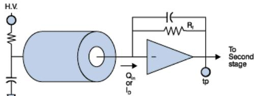
The energy rate limit of RC preamplifiers is a function of feedback resistor value ( $R_f$ ) and dynamic range.
