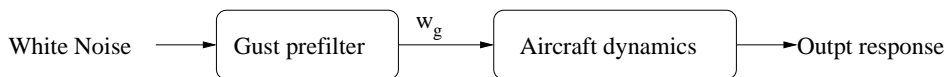
Figure 2. Schematic of the white noise to output mapping used for linear gust analysis.
