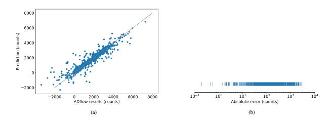
Fig. 11 Validation of  $C_m$ : (a) prediction vs. ADflow results; (b) absolute error.
