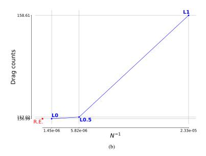
Fig. 5 Grid convergence study: (a) NACA 0012 case which has a convergence order of 10.97; (b) RAE2822 case which has a convergence order of 5.98.
