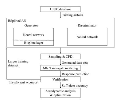
Fig. 1 BSplineGAN-based fast interactive aerodynamic optimization framework.
