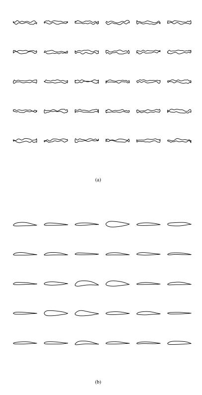
Fig. 8 Comparison between randomly generated shapes using: (a) B-spline curve; (b) BSplineGAN parameterization.
