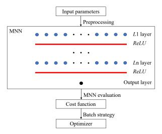
Fig. 4 Construction process of MNN surrogate model.
