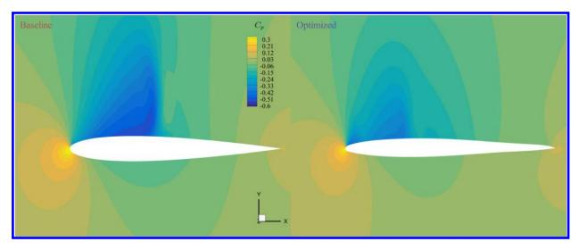
Fig. 13 Comparison of pressure contour between the baseline and optimized designs. The optimized design reduces the shock intensity for drag reduction.
