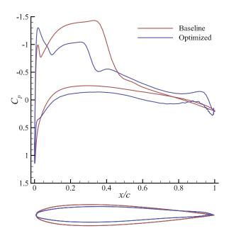
Fig. 12 Comparison of pressure and airfoil profiles between the baseline and optimized designs. The optimized design reduces the shock intensity for drag reduction.
