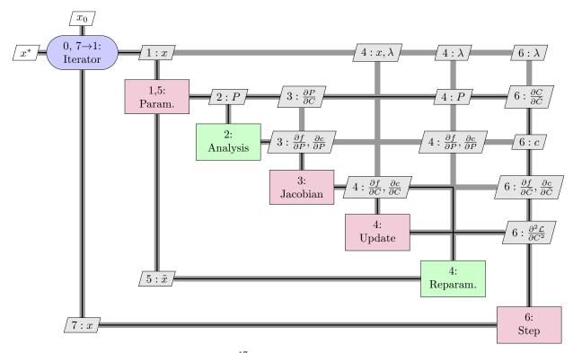
Figure 3: eXtended Design Structure Matrix<sup>17</sup> for the incorporation of the dynamic parametrization scheme.
