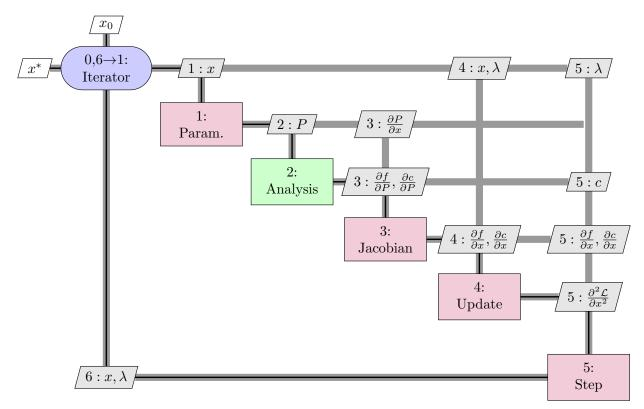
Figure 2: eXtended Design Structure Matrix<sup>17</sup> for quasi-Newton SQP-based shape optimization.
