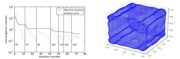
Figure 8: The free-form shape approximation problem in which a sphere morphs into an cube. On the left is the convergence history and on the right is the final shape. In the plot on the left, the small numbers indicate the total number of control points after each reparametrization.
