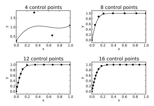
Figure 4: Snapshots of the shape during an adaptive parametrization shape optimization. The curve being approximated is the hyperbolic tangent function. Each snapshot corresponds to the partially converged shape just prior to the next parametrization refinement. Note the x-positions of the control points — a constant arc length condition is used to determine the new locations of the control points for each refinement (the plot is not to scale).
