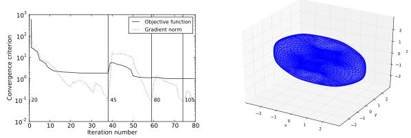
Figure 7: The free-form shape approximation problem in which a sphere morphs into an ellipsoid. On the left is the convergence history and on the right is the final shape. In the plot on the left, the small numbers indicate the total number of control points after each reparametrization.
