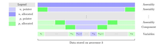
Figure 7: Data storage for the u and p vectors for a Component object and all of the Assembly instances above it in the hierarchy tree.
