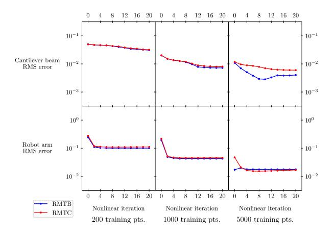
Figure 6: Error versus number of nonlinear iterations for the 3-D cantilever beam and 3-D robot arm problems. The number of iterations after which the improvement plateaus is problem-dependent, but as a general recommendation 10–20 iterations are worthwhile.
