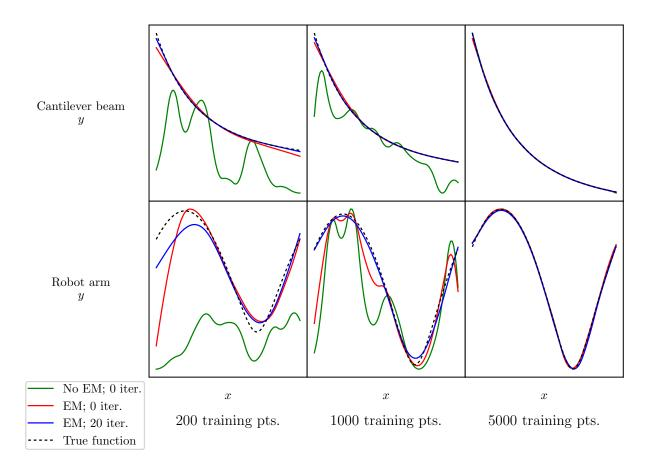
Figure 5: The true function compared to the RMTS interpolant with and without energy minimization and nonlinear iterations. The test problems are the 3-D cantilever beam and 3-D robot arm problems. The conclusion is that energy minimization and nonlinear iterations are both necessary and beneficial for smaller datasets with fewer than  $\mathcal{O}(10^3)$  points.
