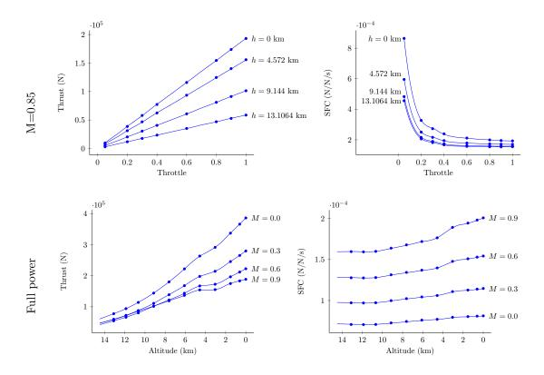
Figure 9: 1-D slices versus throttle (top) and altitude (bottom) for the 3-D aircraft engine model.
