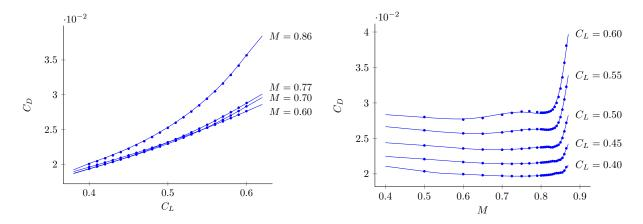
Figure 8: 2-D surrogate model for aircraft aerodynamics with drag coefficient computed as a function of lift coefficient and Mach number.
