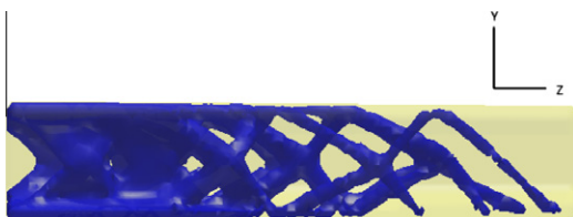
Fig. 20. Span-wise view of the optimized wing structure.
