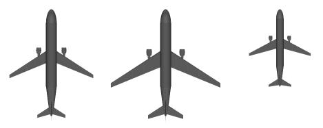
Figure 2. Planform view of LASR (left), A330 (center) and A320 (right)
