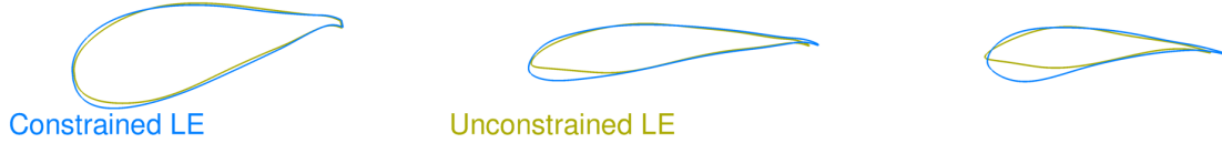
Figure 19: Comparison of airfoil profiles obtained from multipoint optimizations with and without LE geometric constraint.
