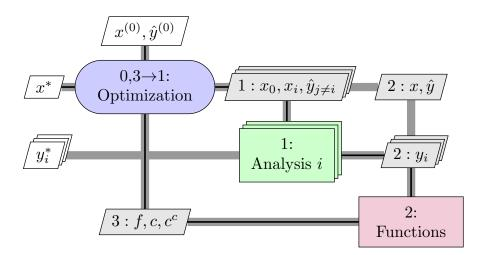
Figure 5. Diagram of the IDF architecture.
