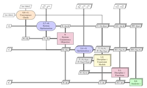
Figure 10. XDSM for the ECO architecture.
