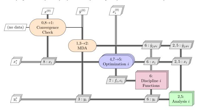
Figure 15. Diagram for the MDOIS architecture.
