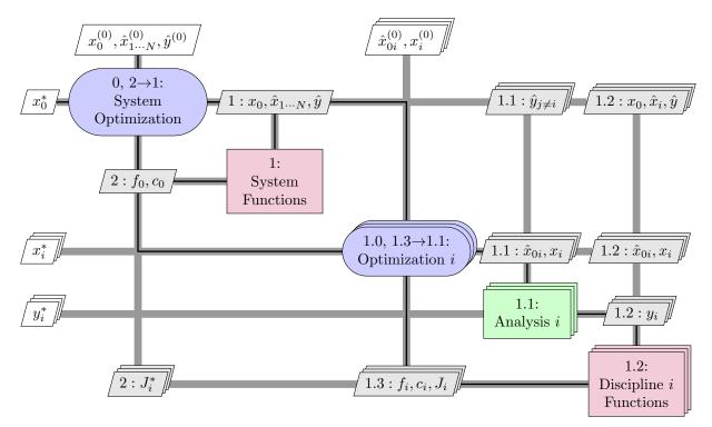
Figure 9. Diagram for the CO architecture.
