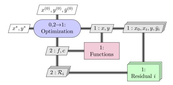
Figure 4. Diagram for the SAND architecture.
