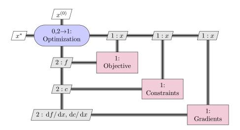
Figure 2. Gradient-based optimization procedure.
