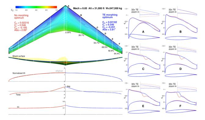
Figure 5: An optimized wing in an off-design condition (left, red), compared to the same wing with trailingedge morphing (right, blue) [LM15].
