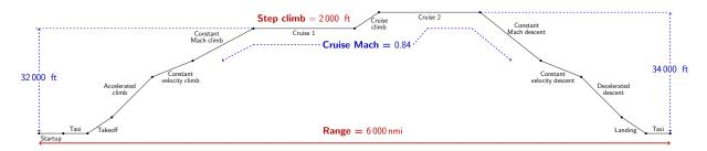
Figure 1: Typical mission profile for a long-range commercial transport aircraft.
