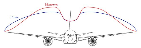
Figure 2: Twist morphing can shift the spanwise lift distribution inboard under critical load conditions to reduce wing structural weight.
