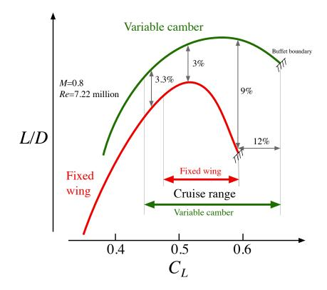
Figure 3: Variable-camber trailing edge increases the aerodynamic performance over a range of lift coefficients (adapted from Ref. [SH98]).
