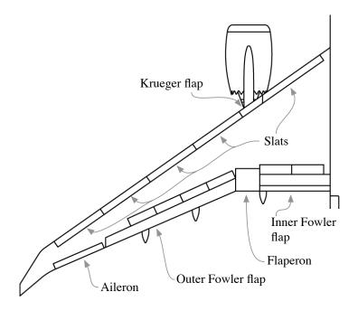
Figure 4: The trailing edge of a modern transport aircraft has either Fowler flaps or ailerons over most of its length.
