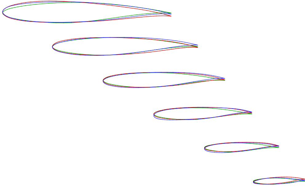
Figure 13: Airfoil shapes for the initial design (green), AMD optimization (blue), and design optimization result (red).
