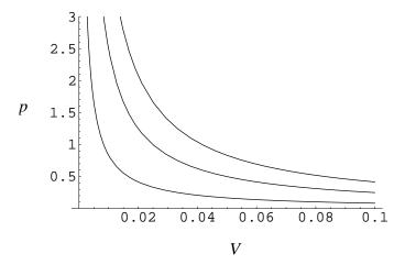
Except at low pressure this is not a very good representation of the behavior of a real gas. A better representation is the van der Waals equation of state:
