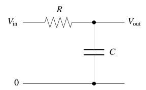
This circuit acts as a low-pass filter: you send a signal in on the left and it comes out filtered on the right.
