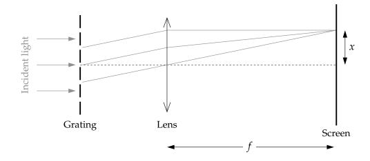
Theory tells us that the intensity of the diffraction pattern on the screen, a distance x from the central axis of the system, is given by
