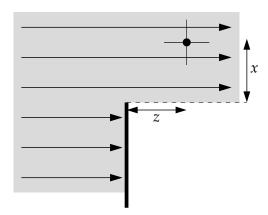
The wave will be diffracted at the edge and the resulting intensity at the position (x, z) marked by the dot is given by near-field diffraction theory to be
