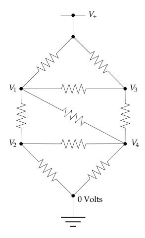
All the resistors have the same resistance R. The power rail at the top is at voltage  $V_+ = 5$  V. The question is, what are the other four voltages,  $V_1$  to  $V_4$ ?
