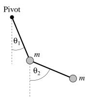
The position of the arms at any moment in time is uniquely specified by the two angles  $\theta_1$  and  $\theta_2$ . The equations of motion for the angles can be derived using the Lagrangian formalism, as follows.
