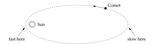
This is a classic example of a system for which an adaptive step size method is useful, because for the large periods of time when the comet is moving slowly we can use long time-steps, so that the program runs quickly, but short time-steps are crucial in the brief but fast-moving period close to the Sun.
