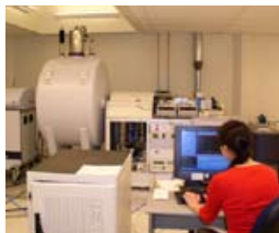
Fourier transform ion cyclotron resonance mass spectrometer (Hakansson)
