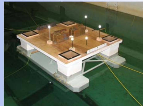
Oil platform awaiting seakeeping testing with infrared camera system passive markers. The camera system tracks a three dimensional model in a defined space.
