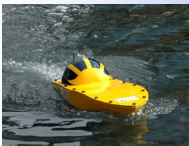
BathyBoat taking measurements in a local lake and demonstrating its autonomous navigation capabilities.
