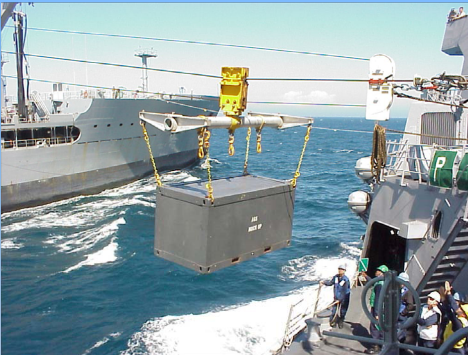
At sea evaluation of replenishing a new ammunition package for a future class of ships. The tests were conducted by the Port Hueneme Division of NAVSEA off the Southern California coast.
