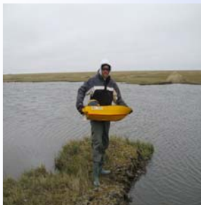
Launching BathyBoat to take bathymeter readings in one of the many lakes on the Northslope of Alaska.
