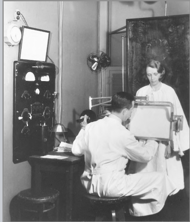
1933 Fluoroscopic System, Mayo Foundation (Schueler BA, Radiographics 2000; 20:1115-1126)
