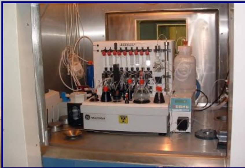
Automated FDG production system (GE Tracerlab) shown within a hot cell (UC Davis).
