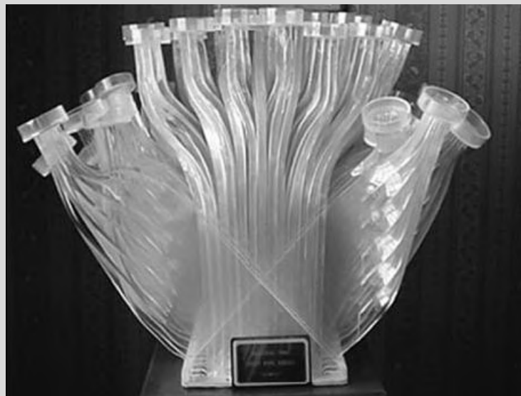
The Baird multi-crystal camera used 293 crystals, 3/8 inch in diameter, arranged in a flat mosaic pattern. Gamma ray event positions were determined using light pipes to each crystal and photomultiplier tubes.
