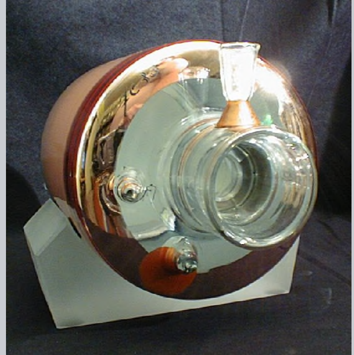
Front and back view of the glass vacuum tube of a Philips x-ray image intensifier.
