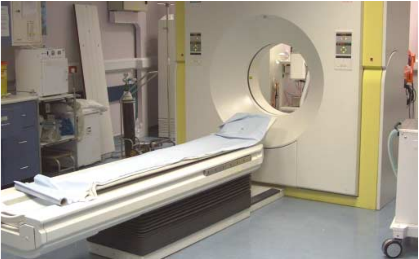
Fig 6 A modern computed tomography scanner. The patient lies on the couch and is moved through the scanner. The x ray tube is behind the cladding, and, as it rotates, it can be quite noisy
