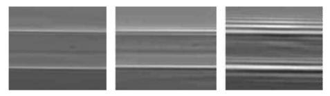
Figure 14: By changing the geometry in coherence-based radiology, one can move from the edge-refraction-enhancement regime (left) to the edge-diffraction-enhancement regime (right). The images show the two edge between different parts of an optical fiber (Ref. 7).
