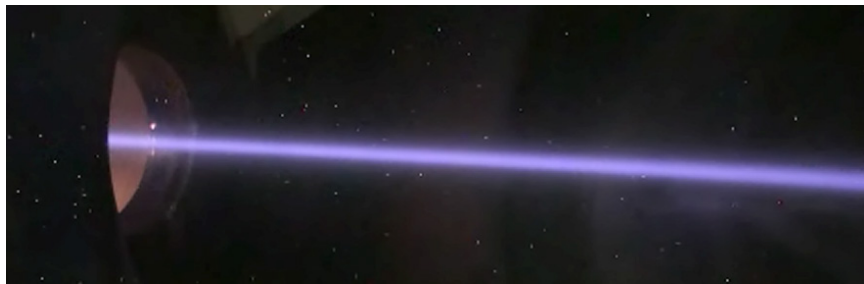
FIGURE 4.6 Photo of a beam of deuterium ions after acceleration in the neutron driver produced for SHINE by Phoenix Nuclear Labs. SOURCE: Courtesy of Phoenix Nuclear Labs.
