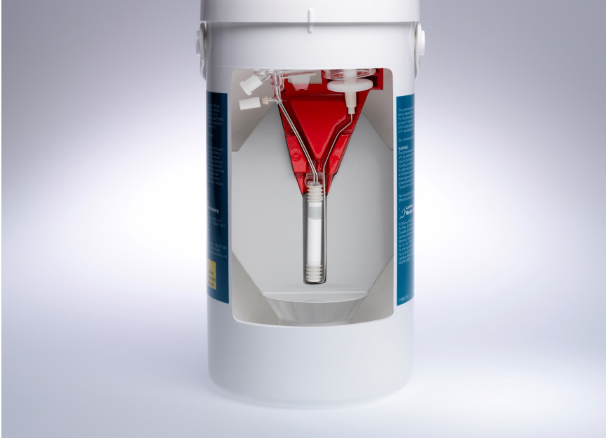
FIGURE 2.6 Internal structure and external view of a Technelife® Tc-99m generator used for obtaining Tc-99m from high-specific-activity Mo-99. The generator (including shielding) is 25 cm in height, 13.2 cm in diameter (14.2 cm at generator top), and weighs 11 kg and 15 kg for a 37-74 GBq and 111-666 GBq activity generator, respectively. A typical generator column (vertical cylinder in center of container) is about 6-8 cm long and about 1.5-2 cm in diameter. The column is enclosed in a radiation-shielded plastic container. SOURCE: Image courtesy of Lantheus Medical Imaging, Inc.
