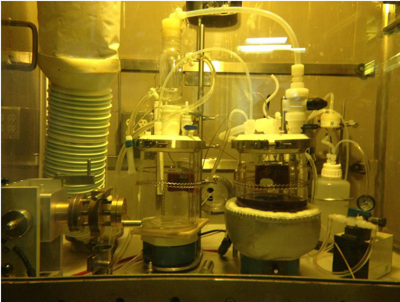
FIGURE 4.3 Top : Hot cells at MURR for processing of Mo-98 targets for North-Star's neutron capture production process. Bottom : Dissolution apparatus in the hot cell. SOURCE: Courtesy of University of Missouri Research Reactor Center.
