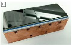
Figure 3. (a) Ge hybrid pixel detector prototype, with a sensor of 256  $\times$  256 pixels (55- $\mu$ m pixel size) bonded to a single Medipix3 readout chip. (b) Larger GaAs hybrid pixel detector, with two sensor tiles of  $768 \times 512$  pixels (each bonded to six Medipix3 chips) mounted on a single circuit board.
