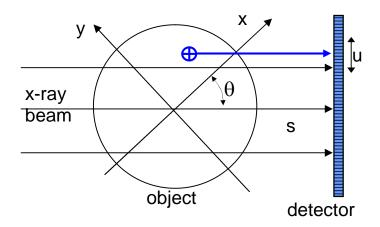
The variable u describes the projection position in the detector,  $\theta$  describes the amount of the rotation of the object about the cylindrical axis, and S describes the path length of the beam through the object. For projections contained in a transaxial plane, projection values as a function of  $\mu$  and  $\theta$  are given by the Radon transform<sup>3</sup>,
