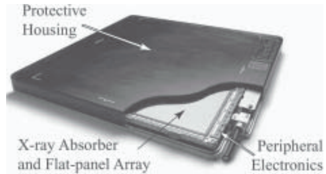
Figure 3. Configuration of a DR detector that is based on an a-Si:H flat-panel array, showing the protective housing, the x-ray absorber (in this case, a-Se) in direct contact with the flat-panel array, and the peripheral electronics on the edge of the glass substrate. (Image courtesy of K. Schwartz, Direct Radiography Corp, Newark, Del.)
