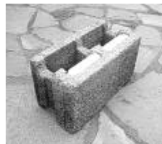
Figure 70: Wood waste at the University of Idaho chipper facility could be recycled into building materials similar to this Faswall wall-form block, which is manufactured from waste wood and cement.
