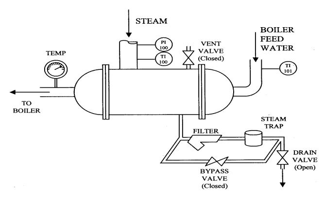
Condensate is withdrawn through a thermodynamic steam trap at the bottom of the shell. The water flows once through the 3/4" nominal tubes. There are 1000 tubes. "When the system was put into operation 3 hours ago everything worked fine," says the supervisor. "Now, however, the exit boiler feed water is 42°C instead of the design value. What do we do? This difficulty is costing us extra fuel to vaporize the water at the boiler." Fix it.
