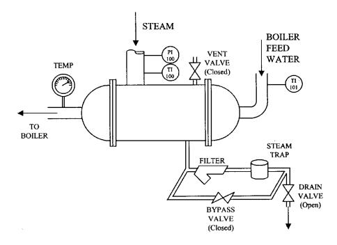
$$T_{out} = T_{steam} - (T_{steam} - T_{in}) \exp(-UA/mC_P)$$
