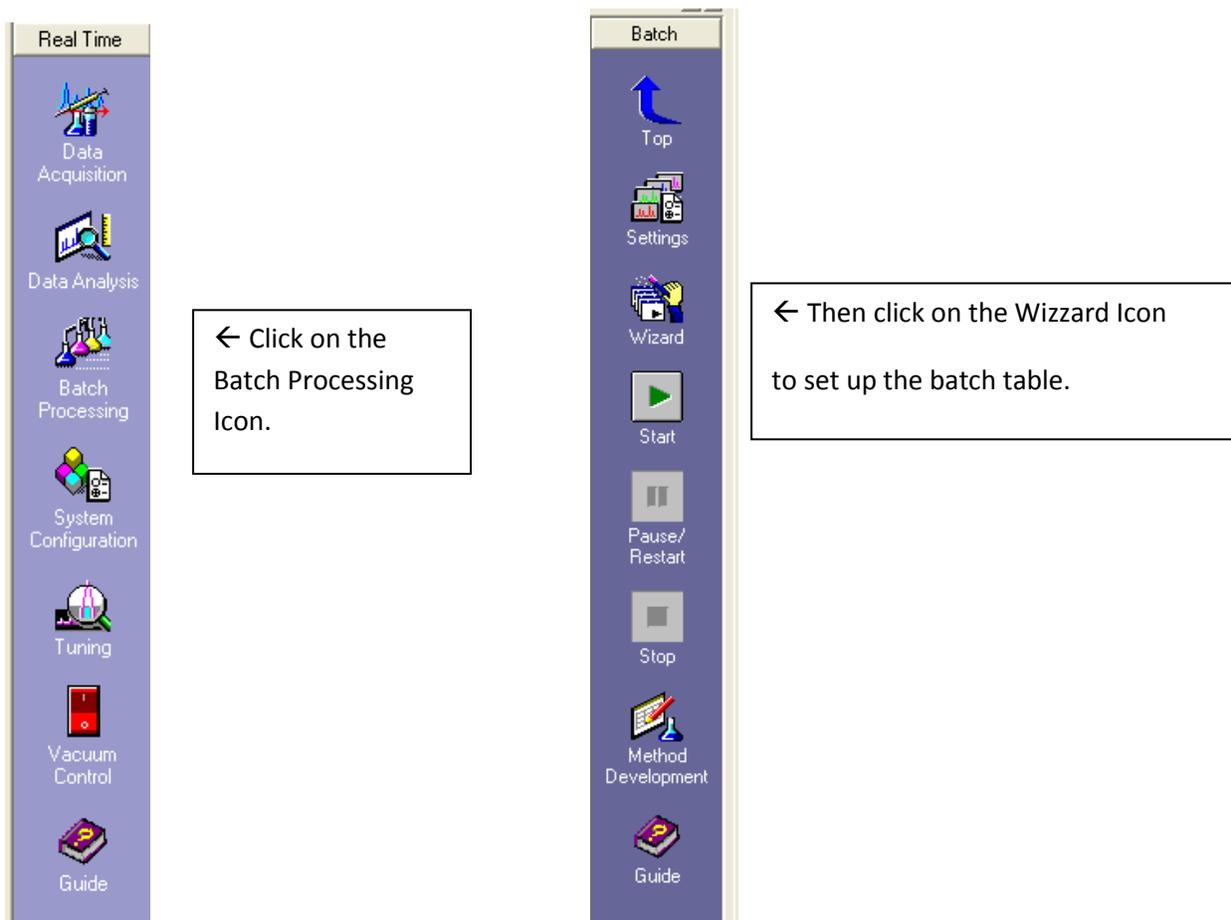
After the batch table has been set up, put your samples into the auto-sampler carousel, and click on the Start icon to start the batch.
