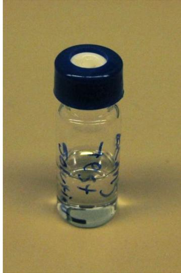
The minimum volume of solution is 450  $\mu$ l. If you cannot spare that much solution, you can use a conical glass insert in the vial, so that the solution level will be high enough for the syringe needle to enter it.
