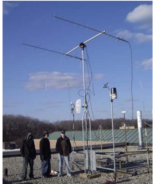
Part of the EECS 430 team and the newly constructed 2m/70cm circularly polarized, tracking antenna system for amateur space communication.
