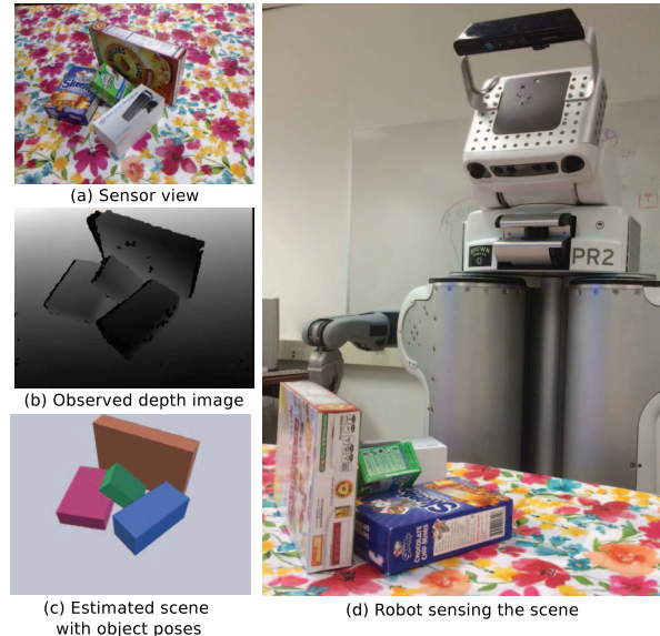
Fig. 1: A physically plausible scene estimate of a cluttered environment (a) viewed by a PR2 robot for manipulation. Using a Bayesian particle filter, hypotheses of possible states are generated through sampling, projected into physical plausible states and evaluated against robot's observation (b) to infer the most likely scene state (c) for manipulation.
