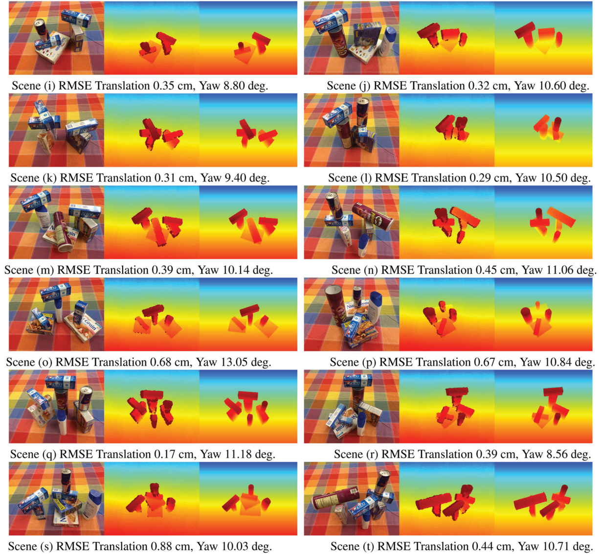
Fig. 7. Pose estimation results for known axiom sets in scenes containing five to seven objects. Each subfigure, shows the RGB (left) and depth (middle) from a RGBD camera mounted on the head of the PR2 and estimated scene graph as a depth image (right), as well as the RMSE for translation and rotation error.
