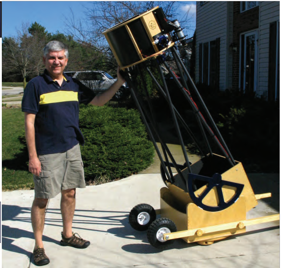
Here's Doug Scobel with his "completed" 16-inch f/4.6 AstroSystems TeleKit. But is it really done?
