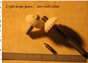
Gear Manufacture: The gear manufacturing was accomplished using my small milling machine and metal lathe using Delrin plastic and carbon loaded - fiber glass filled nylon material for the gears. A 4 inch diameter 72:1 rotary table was also used for proper gear tooth spacing.
