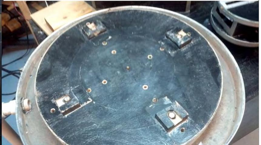
Wa La , the mirror is always in the center of the turntable and in the same spot. Before placing the mirror on the table, I put down a cushion for a soft support for the mirror (*see picture below*) and adjust the height of the acorn nut just enough so the mirror hole can find it but not resting on it. The cushion is cut from a cheap thin yoga mat.
