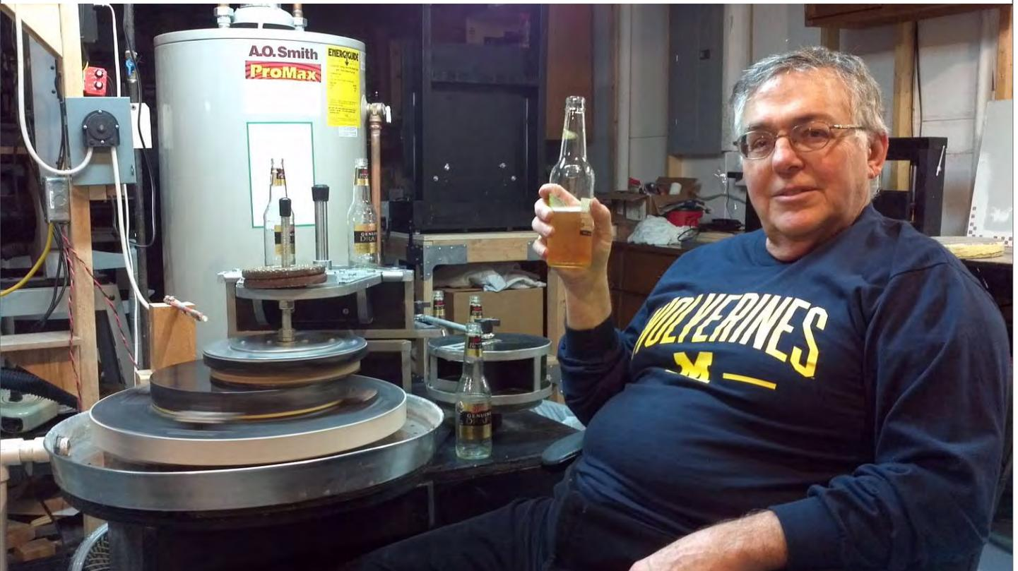
Polishing is quite easy because I don't have to sit there. I made a cerium dispensing system consisting of a tank, a peristaltic pump and an on-off timed relay. Polishing out a 12" blank takes three to five hours, after which initial testing can be done. I use the Ronche test at this point.
