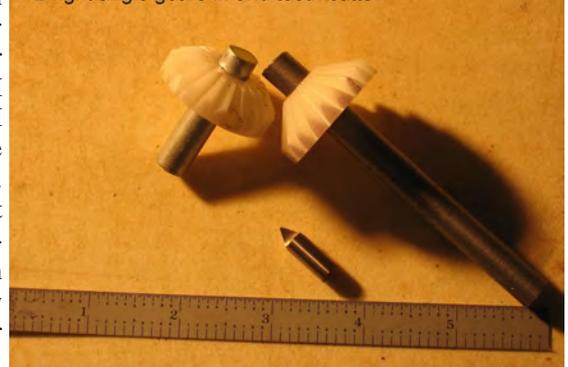
**Gear Manufacture:** The gear manufacturing was accomplished using my small milling machine and metal lathe using Delrin plastic and carbon loaded - fiber glass filled nylon material for the gears. A 4 inch diameter 72:1 rotary table was also used for proper gear tooth spacing.
