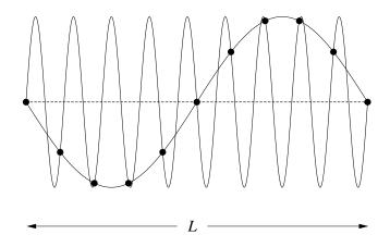
It depicts a one-dimensional version of the aliasing problem. The dots are atoms. The solid lines represent two possible waves, both of which correspond to the same positions of the atoms.
